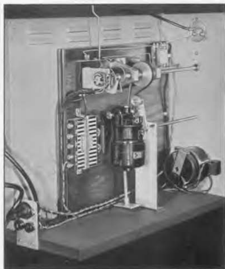
Figure 2. Rear view, showing the motor drive and frequency-sweeping capacitor.
