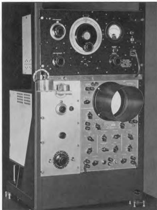
Figure 1. Panel view of the crystal mode indicator.
